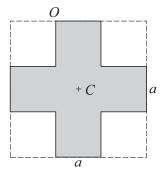
A uniform lamina of mass M is in the shape of a square of side 3a from which the four corner squares of side a have been removed (see diagram). Show that its moment of inertia about an axis through its centre C, perpendicular to its plane, is  $\frac{29}{30}Ma^2$ . [5]
