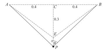
The particle is released from rest at a point vertically below E. Its distance below E at time t s after release is x m, where x is small (see diagram). Show that, if  $x^2$  and higher powers of x are neglected, the tension in each of the strings AP and BP is 10(1+6x) N, and that each string makes an angle  $\theta$  with the vertical, where  $\cos \theta = 0.6 + 1.28x$ .
